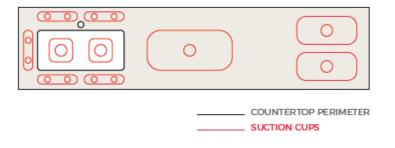
Internal holes: Atlas Plan recommends using a waterjet or CNC contouring machine. Circular holes are made using wet diamond core bits. Abundant water flow is required both internally and externally to the cutting circumference.
